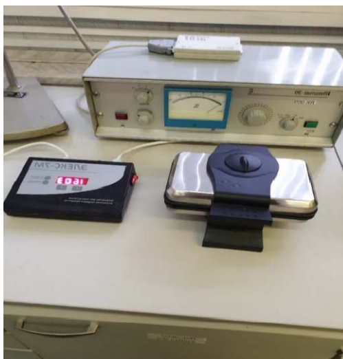
Figure 4 Device used for determining the humidity of food raw materials and products Eleks – 7M, Russian Federation, Moscow (Manufacturer Limited Liability Company "Tagler").
