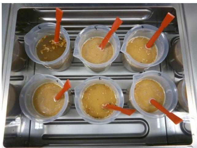
**Figure 2** Mashing in laboratory in water-bath thermostat
