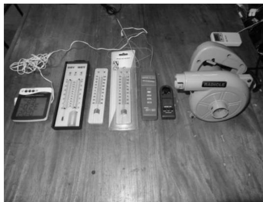
**Figure 5** Photographic view of data measuring instruments: (a) Data logger (b) Digital thermometer, hygrometer, anemometer, and blower.
