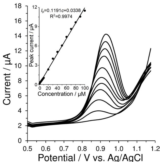
**Figure 6** Voltammograms for 0, 10, 20, 30, 40, 50, 60, 70, 80, 90, and 100  $\mu\text{M}$  cholecalciferol with corresponding calibration curve obtained at GCE. Measured by DPV at  $E_{\text{step}} = 5 \text{ mV}$ ,  $E_{\text{ampl}} = 140 \text{ mV}$ ,  $t_{\text{int}} = 0.5 \text{ s}$ , and  $v = 50 \text{ mV}\cdot\text{s}^{-1}$ .
