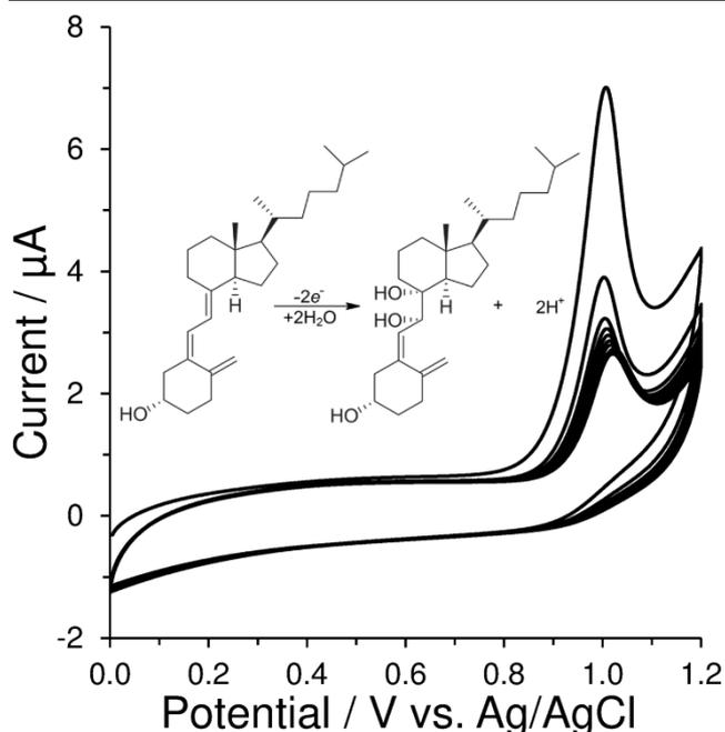
**Figure 3** Repetitive cyclic voltammetry (10 cycles) of 0.2 mM cholecalciferol at GCE performed in 50% ethanol containing 0.1 M LiClO<sub>4</sub> at 50 mV·s<sup>-1</sup>.
