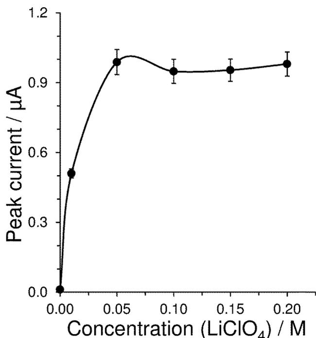
**Figure 5** Dependency of peak current on amount of LiClO<sub>4</sub> in supporting electrolyte containing always 50% ethanol. For concentration of 100 μM cholecalciferol measured at GCE by DPV at *E<sub>step</sub>* = 5 mV, *E<sub>ampl</sub>* = 25 mV, *t<sub>int</sub>* = 0.5 s, and *v* = 50 mV·s<sup>-1</sup>.
