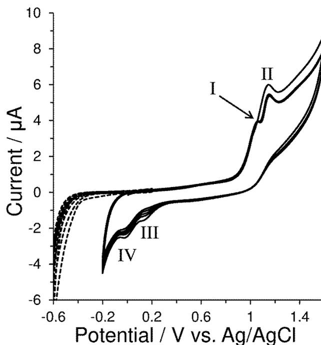
Figure 2 Cyclic voltammetry of 0.5 mM cholecalciferol at PtE performed in 98% ACN containing 0.1 M  $\text{LiClO}_4$  at  $50 \text{ mV} \cdot \text{s}^{-1}$ .
