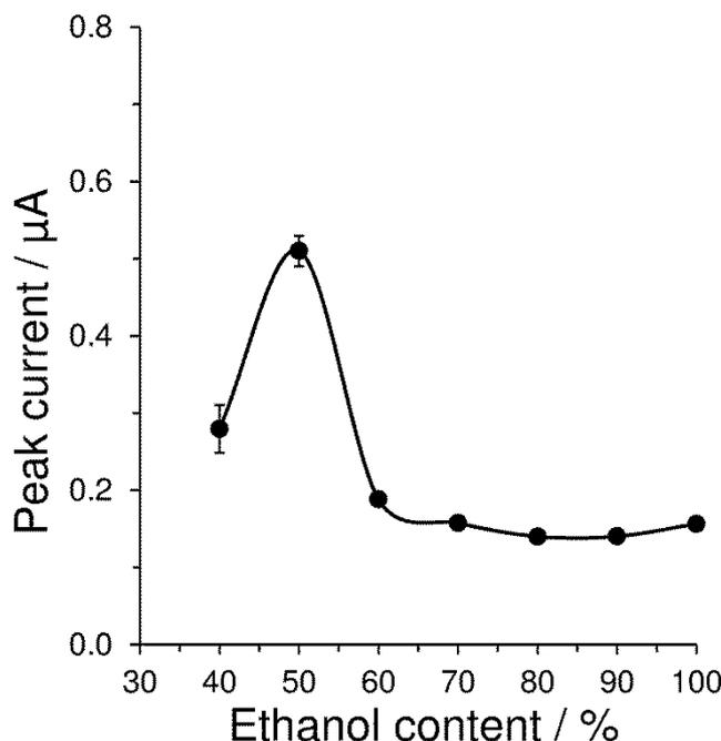
**Figure 4** Dependency of peak current on amount of ethanol in supporting electrolyte containing always 0.1 M LiClO<sub>4</sub>. For concentration of 100 μM cholecalciferol measured at GCE by DPV at *E<sub>step</sub>* = 5 mV, *E<sub>ampl</sub>* = 25 mV, *t<sub>int</sub>* = 0.5 s, and *v* = 50 mV·s<sup>-1</sup>.
